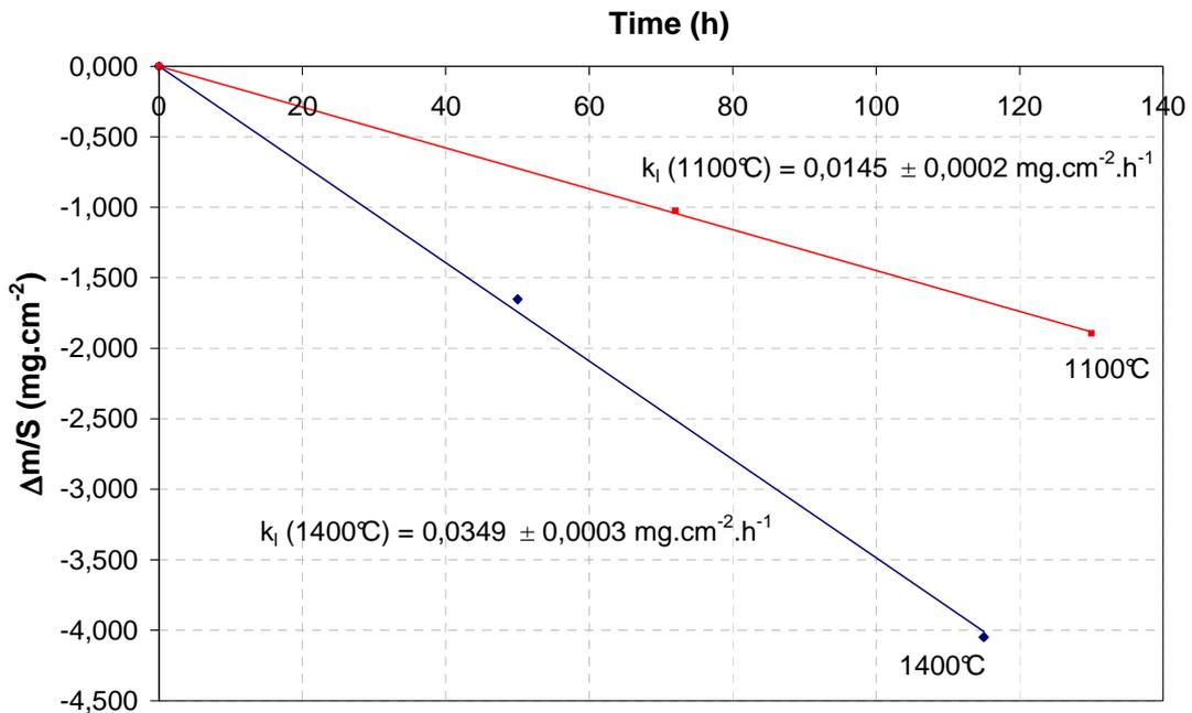
Fig. 2: Weight losses during volatilization of  $SiO_2$  at different temperatures (under corrosion at 50 kPa  $H_2O$ , at  $P_{atm}$  with  $v_{gas} = 5 \text{ cm}\cdot\text{s}^{-1}$ )
