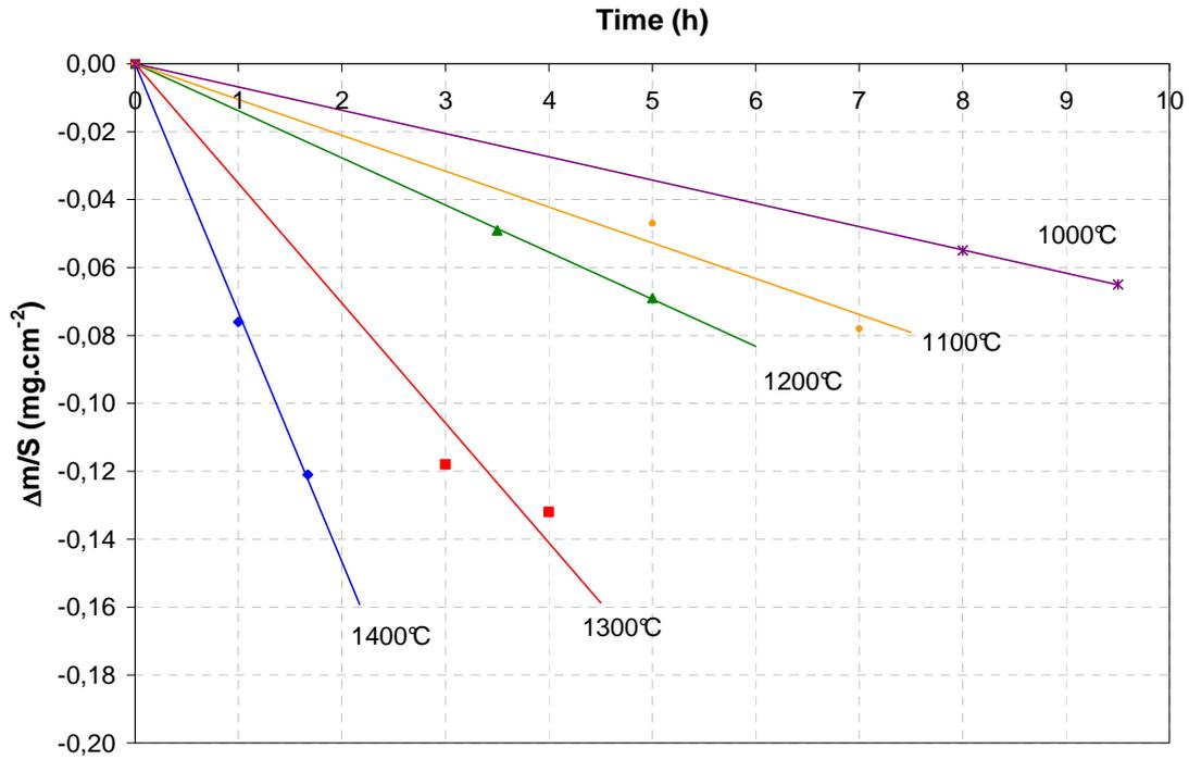
Figure 3: Weight changes during volatilization of  $\text{Sc}_2\text{O}_3$  at different temperatures, under corrosion with 50 kPa  $\text{H}_2\text{O}$ , at  $P_{\text{atm}}$  with  $v_{\text{gas}} = 5 \text{ cm}\cdot\text{s}^{-1}$
