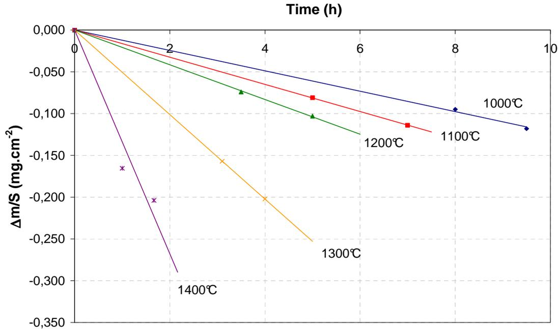
Fig. 4: Weight losses as a function of time during volatilization of  $\text{Y}_2\text{O}_3$  at different temperatures (under corrosion at 50 kPa  $\text{H}_2\text{O}$ , at  $P_{\text{atm}}$  with  $v_{\text{gas}} = 5 \text{ cm.s}^{-1}$ )
