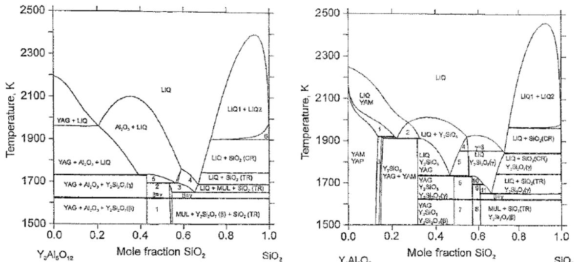
Fig. 8. The phase diagram of the  $Y_3Al_5O_{12}-SiO_2$  system. 1:  $Al_2O_3 + Y_2Si_2O_7(\beta) + MUL$ , 2:  $Al_2O_3 + Y_2Si_2O_7(\gamma) + MUL$ , 3:  $Y_2Si_2O_7(\gamma) + MUL + LIQ$ , 4:  $MUL + LIQ$ , 5:  $Al_2O_3 + Y_2Si_2O_7(\gamma) + LIQ$ , 6:  $LIQ1 + LIQ2 + SiO_2(CR)$ .
