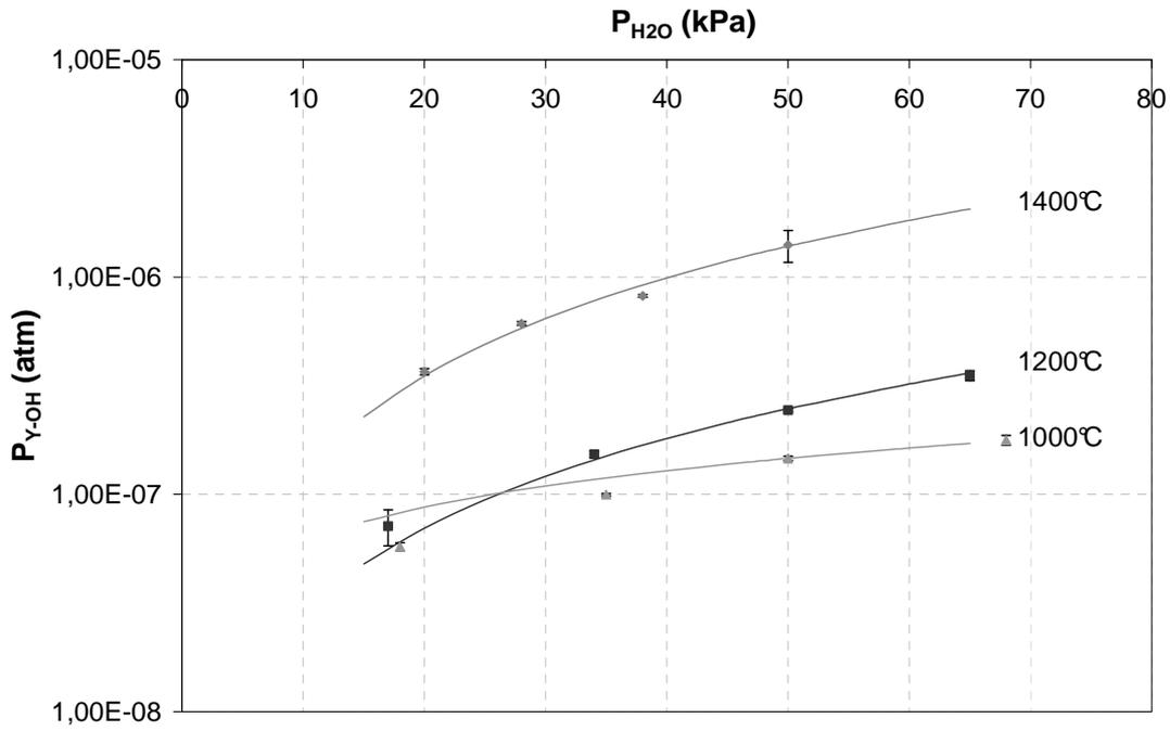
Fig. 9: Comparison of  $P_{Y-OH}$  between calculations (line) (from assessed thermodynamic data) and experience (dots) from volatilization tests at 1000, 1200 and 1400°C under a moist environment ( $P_{tot} = 100$  kPa,  $v_{gas} = 5$  cm.s<sup>-1</sup>).
