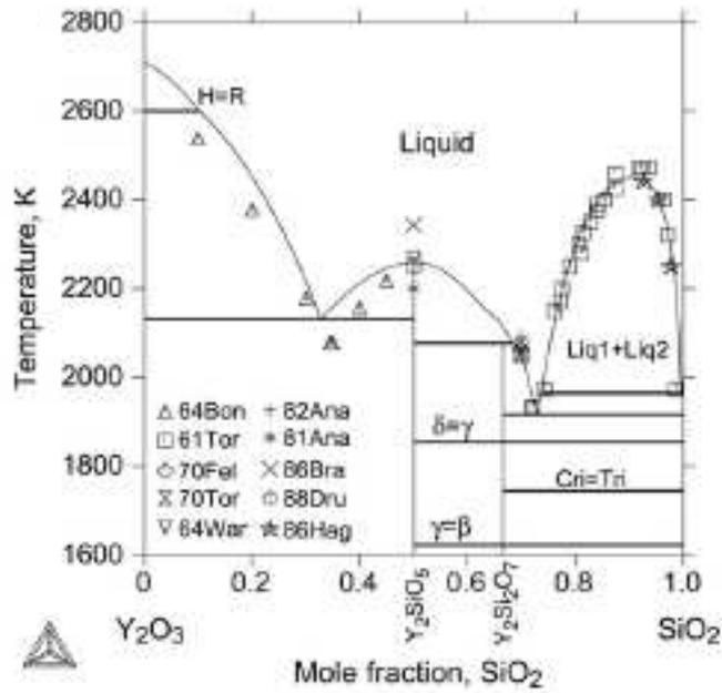
Figure 1: Y<sub>2</sub>O<sub>3</sub>-SiO<sub>2</sub> phase diagram [7].
