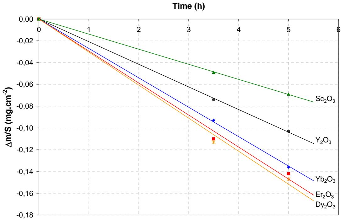
Figure 4: Weight changes during volatilization of  $\text{RE}_2\text{O}_3$  at 1200°C, under corrosion with 50 kPa  $\text{H}_2\text{O}$ , at  $P_{\text{atm}}$  with  $v_{\text{gas}} = 5 \text{ cm}\cdot\text{s}^{-1}$
