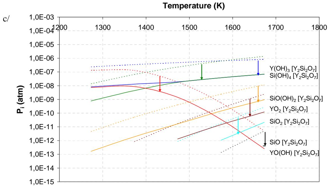
Figure 5: Stability of a/ Y<sub>2</sub>SiO<sub>5</sub> ; b/ Y<sub>2</sub>SiO<sub>5</sub> + Y<sub>2</sub>Si<sub>2</sub>O<sub>7</sub> ; c/ Y<sub>2</sub>Si<sub>2</sub>O<sub>7</sub> revealed through the variation of partial pressures of different gaseous species formed under a moist environment
