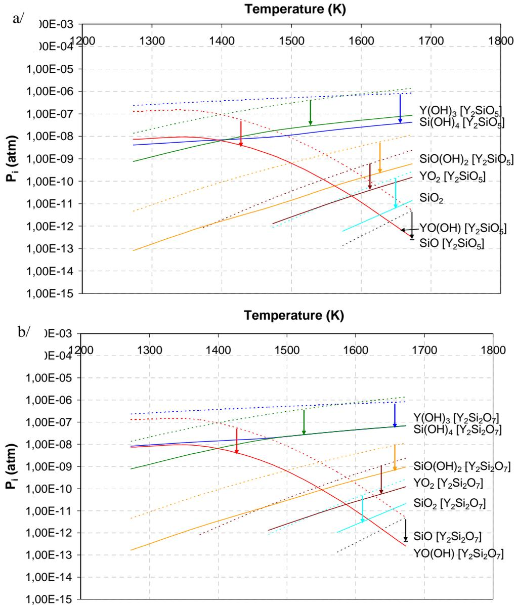
Figure 2. Partial pressures of gaseous species in equilibrium with a/  $Y_2SiO_5$  and b/  $Y_2Si_2O_7$  in a moist environment calculated with Gemini2 ( $n_{Ar} = 0.4$  mol;  $n_{O_2} = 0.1$  mol and  $n_{H_2O} = 0.5$  mol)
