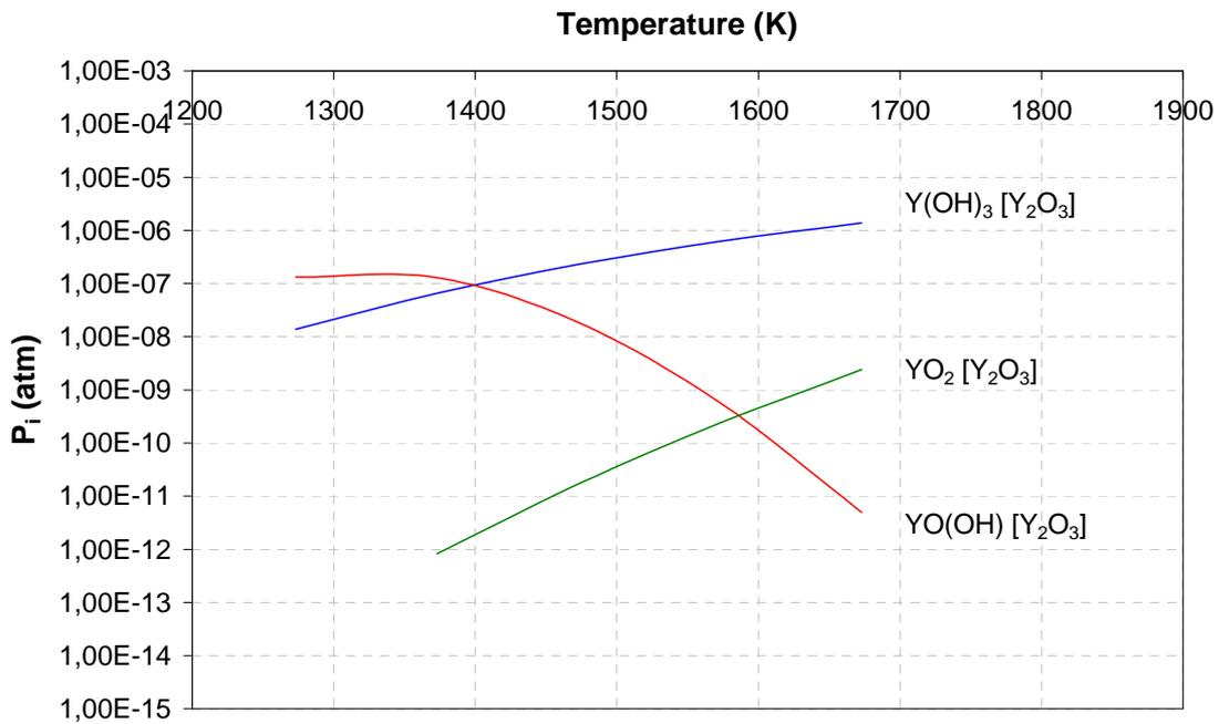
Fig. 8: Partial pressures of  $Y(OH)_3$ , YOOH and  $YO_2$  over  $Y_2O_3$  at equilibrium in a moist environment (calculated with the assessed thermodynamic data of  $Y(OH)_3$  and YOOH) ( $P_{Ar} = 40$  kPa,  $P_{O_2} = 10$  kPa,  $P_{H_2O} = 50$  kPa).
