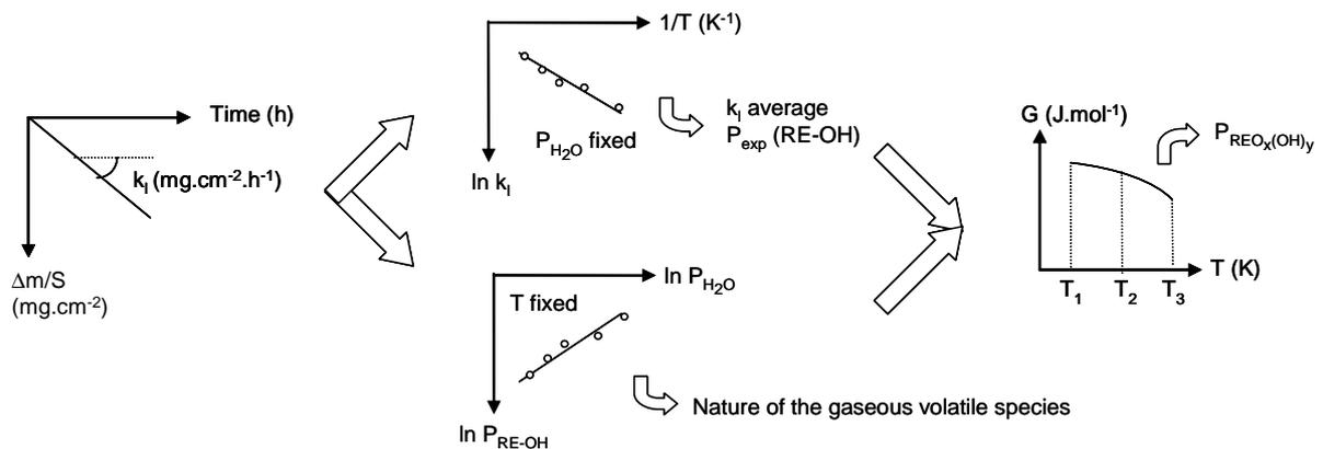
Figure 2: Experimental approach used for the assessment of the hydroxide thermodynamic data.
