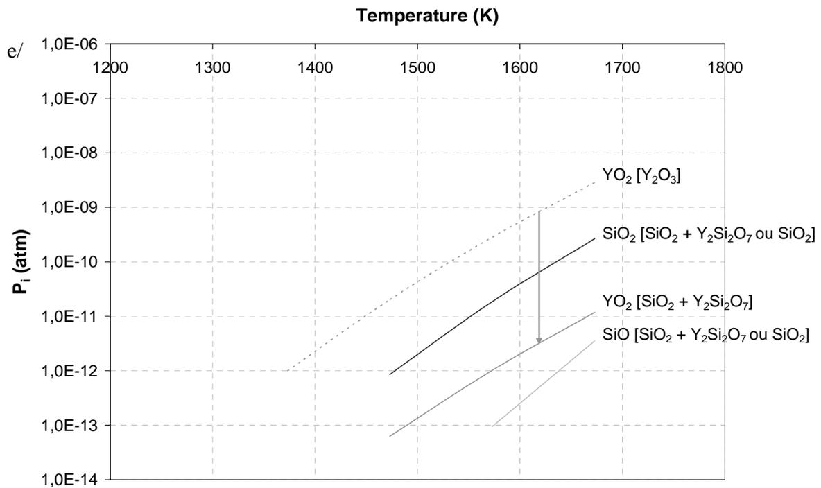
Figure 4 : Stability of a/  $Y_2Si_2O_7$  ; b/  $Y_2SiO_5 + Y_2Si_2O_7$  ; c/  $Y_2SiO_5$  d/  $Y_2O_3 + Y_2SiO_5$  and e/  $Y_2Si_2O_7 + SiO_2$  revealed through the variation of partial pressures of different gaseous species formed under air.
