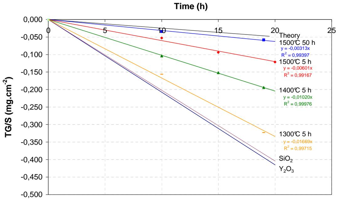
Figure 4. Weight losses of  $Y_2Si_2O_7$  during corrosion at  $1200^\circ\text{C}$  ( $P_{H_2O} = 50 \text{ kPa}$ ,  $P_{tot} = P_{atm}$ ,  $v_{gas} = 5 \text{ cm.s}^{-1}$ ).
