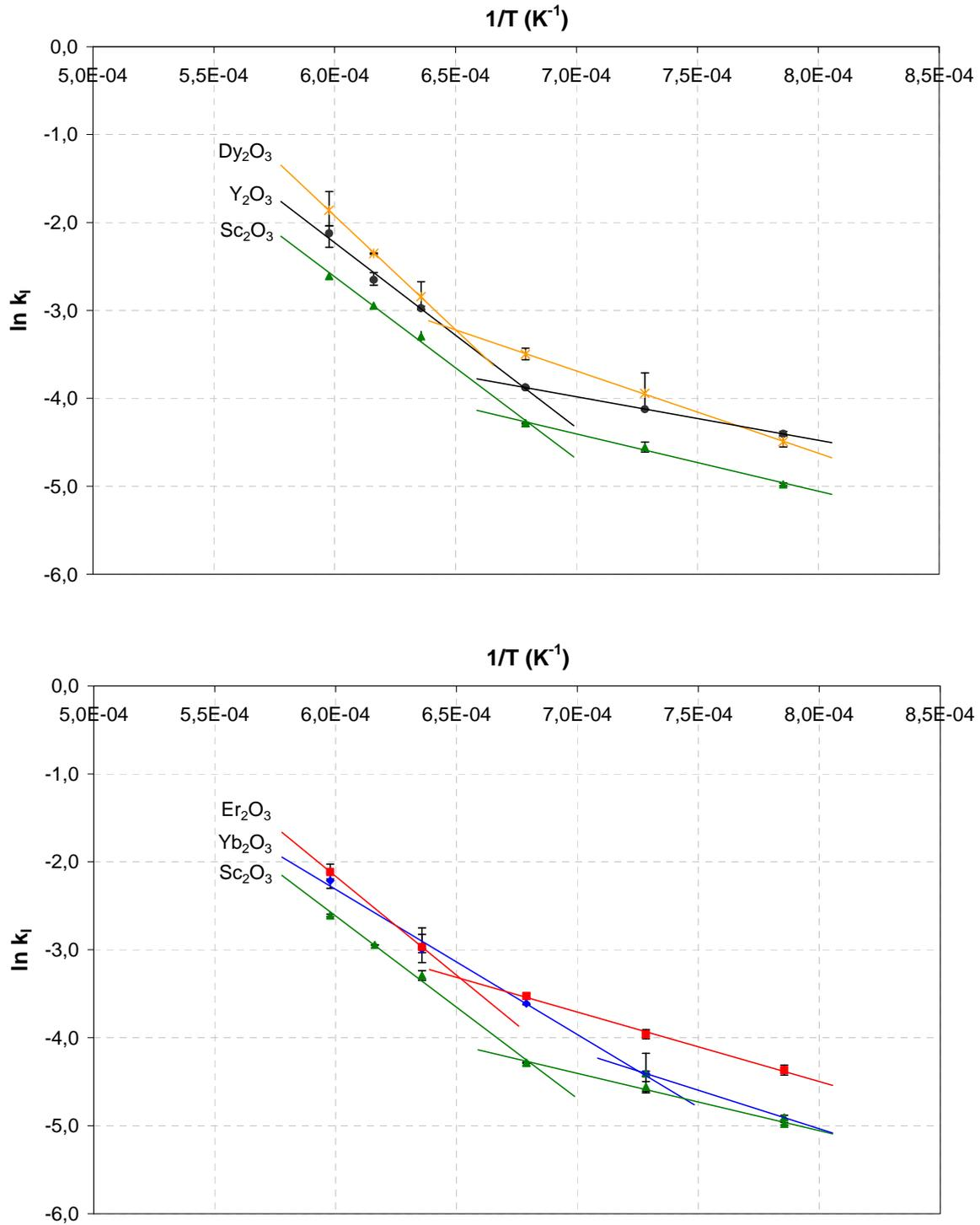
Figure 5: Arrhenius graph concerning the volatilization of the rare earth oxide under a moist environment at high temperature ( $P_{H_2O} = 50$  kPa,  $P_{tot} = P_{atm}$ ,  $v_{gaz} = 5$  cm.s $^{-1}$ ;  $k_1$  in mg.cm $^{-2}$ .h $^{-1}$ ).
