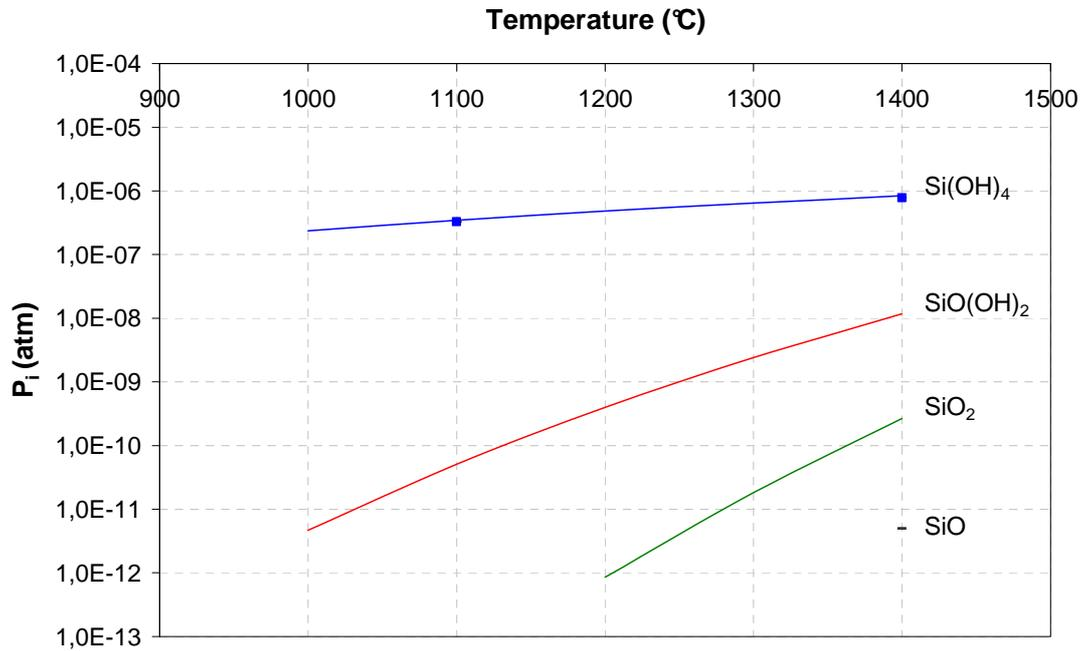
Fig. 1: Theoretical partial pressures of silicon hydroxides in function of temperature. Comparison with experiments : dots (50 kPa  $H_2O$ , at  $P_{atm}$  with  $v_{gas} = 5 \text{ cm}\cdot\text{s}^{-1}$ ).
