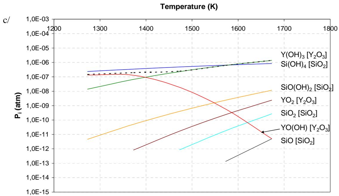
Figure 2 : Stability of  $Y_2O_3$  and  $SiO_2$  revealed through the variation of partial pressures of different gaseous species formed under a/ argon, b/ air ( $n_{Ar} = 0,8$  mol,  $n_{O_2} = 0,2$  mol) ; c/ a moist environment ( $n_{Ar} = 0,4$  mol,  $n_{O_2} = 0,1$  mol and  $n_{H_2O} = 0,5$  mol).
