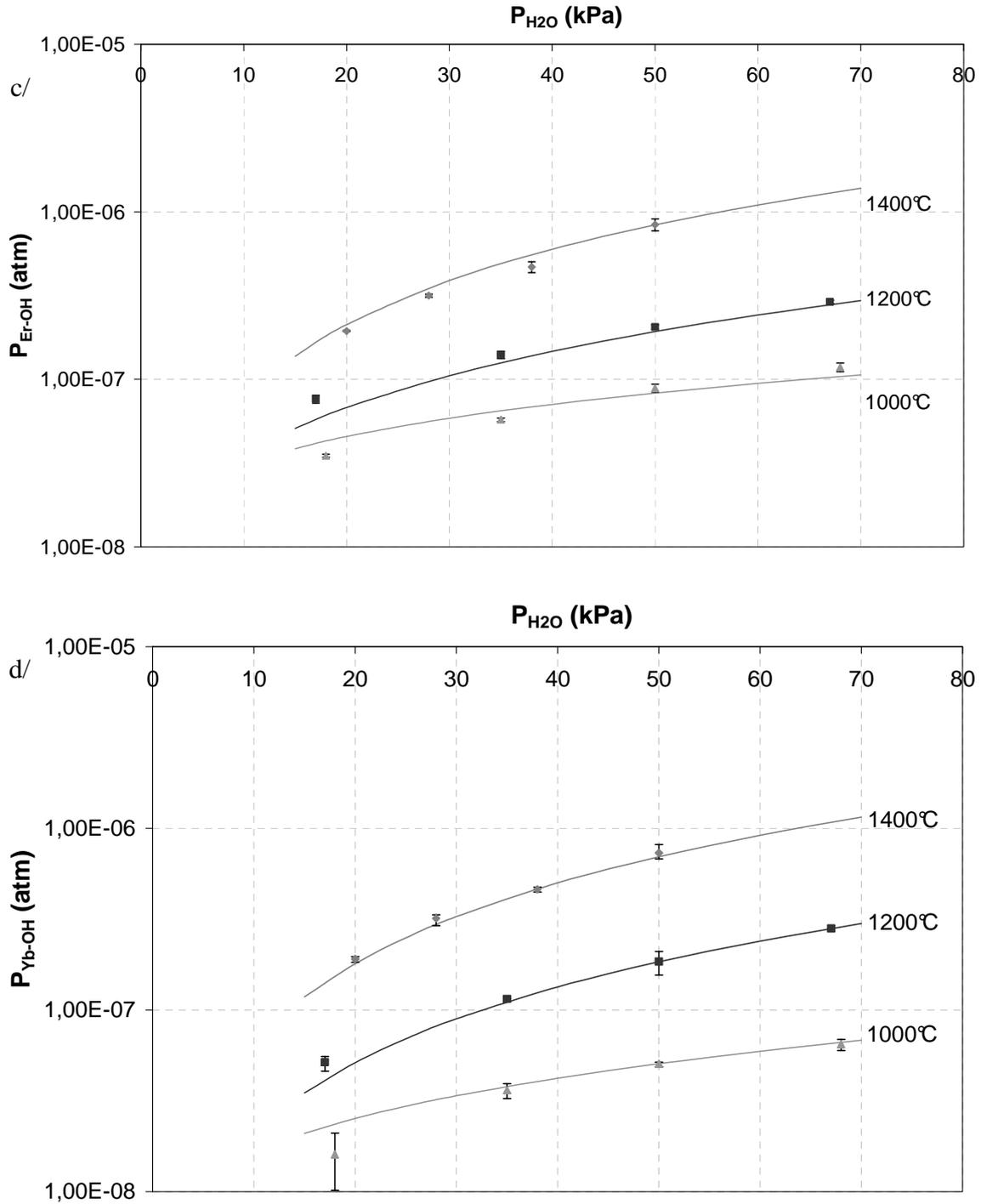
Figure 6: Comparison of experimental (symbols) and calculated (curves) hydroxides pressures using the Gibbs free energies of a/  $Sc(OH)_3$  and  $ScOOH$  formation ; b/  $Dy(OH)_3$  and  $DyOOH$  formation ; c/  $Er(OH)_3$  and  $ErOOH$  formation and d/  $Yb(OH)_3$  and  $YbOOH$  formation ( $P_{tot} = P_{atm}$ ,  $v_{gaz} = 5 \text{ cm.s}^{-1}$ ).
