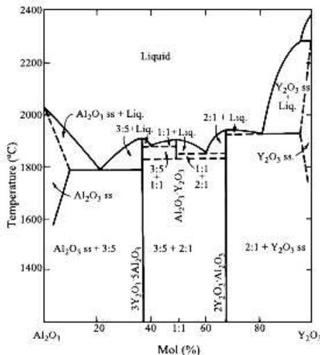
**Figure 2.9** : Diagramme de phases Al<sub>2</sub>O<sub>3</sub>-Y<sub>2</sub>O<sub>3</sub> [Toropov 1972].
