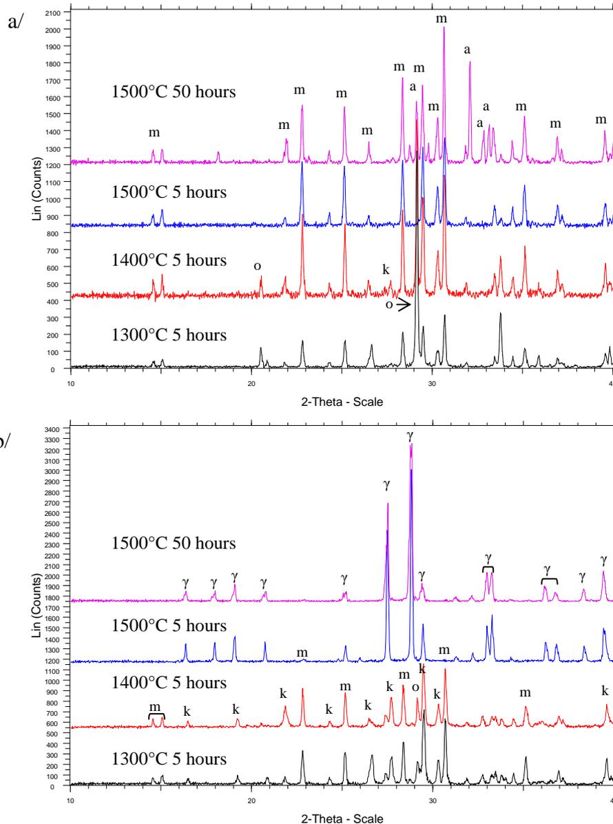
Figure 3. Influence of the sintering conditions on the crystallization degree of a/  $Y_2SiO_5$ ; b/  $Y_2Si_2O_7$  (m =  $Y_2SiO_5$ , o =  $Y_2O_3$ , a = apatite  $Y_{4.67}(SiO_4)_3O$ , k = Keiviite –  $Y_2Si_2O_7$ ,  $\gamma$  =  $\gamma$ - $Y_2Si_2O_7$ ).
