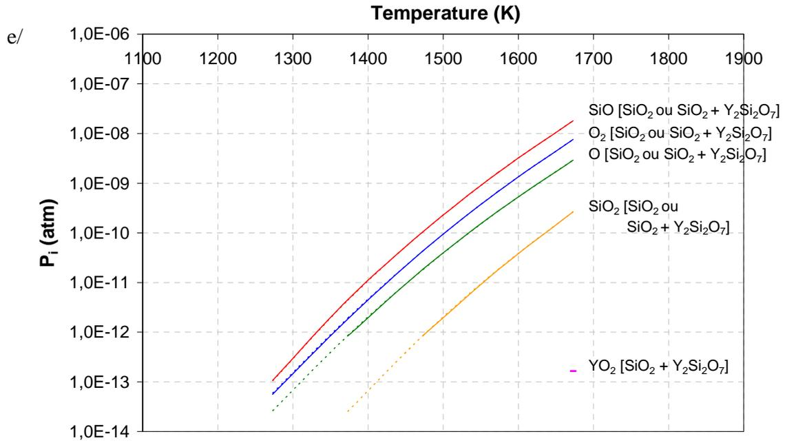
Figure 3 : Stability of a/  $Y_2O_3 + Y_2SiO_5$  ; b/  $Y_2SiO_5$  ; c/  $Y_2SiO_5 + Y_2Si_2O_7$  ; d/  $Y_2Si_2O_7$  ; e/  $Y_2Si_2O_7 + SiO_2$  revealed through the variation of partial pressures of different gaseous species formed under argon.
