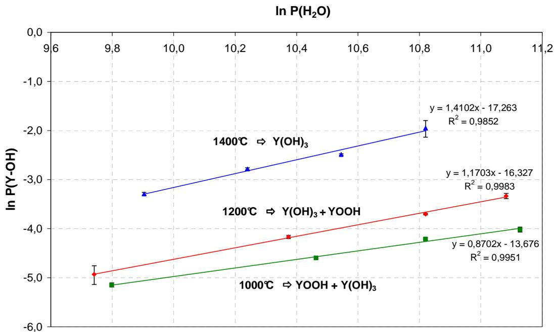
Fig. 6: Determination of the nature of the gaseous species at 1000, 1200 and 1400°C through the extraction of the reaction order associated to  $H_2O$  ( $P_{atm}$ ,  $v_{gaz} = 5 \text{ cm} \cdot \text{s}^{-1}$ ) (with  $P$  in Pa).
