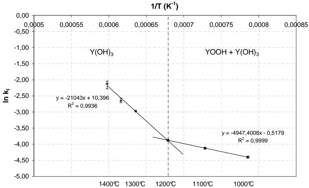
Fig. 5: Determination of the apparent kinetic laws of  $Y_2O_3$  volatilization by reaction with  $H_2O$  (with  $k_1$  in  $mg \cdot cm^{-2} \cdot h^{-1}$ ) (uncertainties are in dots at low temperatures).
