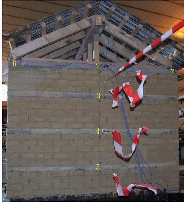
Figure 9.6: Positions of the cable sensors on the North wall of the reduced scale houses
