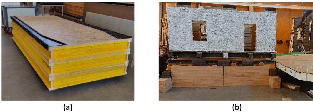
Figure 9.4: Installation of the samples on the shaking table: (a) the wood platform ; (b) specimen with RC bands during the transfer to the shaking table
