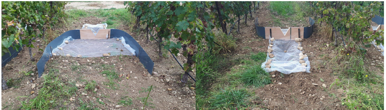
Figure III. 2. Experimental setup installed at the end of the six interrows used for the experimentation. The setup is composed of a calibrated wooden weir equipped with PVC panels redirecting runoff towards the weir, and nets laid on the ground to facilitate sediment recovery for further analyses. Water level sensors were placed parallel to the weirs on the side facing the slope.
